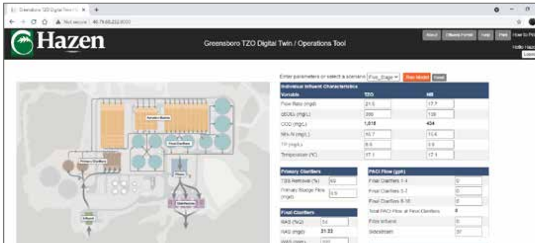
An example dashboard and a photo of staff using the process advisory digital twins for evaluating treatment decisions and testing various operational scenarios.
